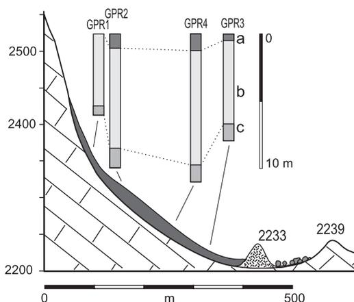
Fig. 7. Internal structure of the Jou Negro ice patch from GPR soundings. (a) mixed layer of ice, snow and clasts, (b) banded glacial ice, (c) clastic layer with glacier ice, detrital material, till and flowing melt water.
