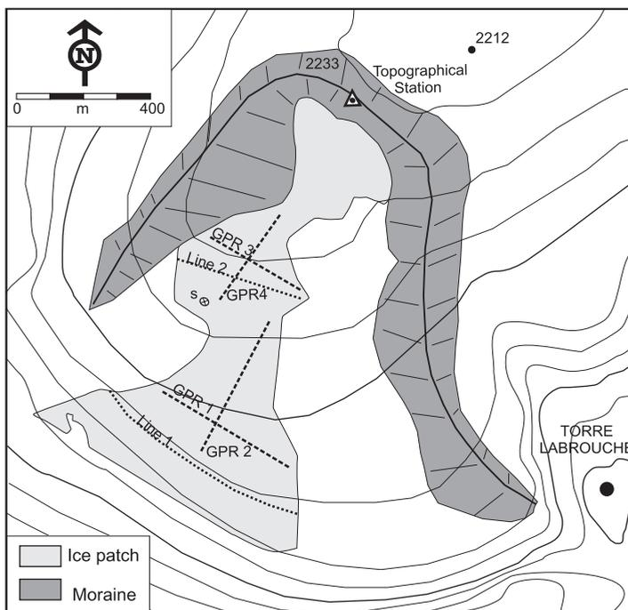
Fig. 4. Location of geodetic control lines (line 1 and 2) and GPR sounding (GPR 1, 2, 3 and 4) in the Jou Negro ice patch. S, mechanical sounding in a moulin.
